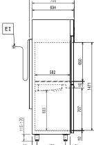
El = Electrical inlet (power) RI = Refrigerant Inlet RO = Refrigerant Outlet
